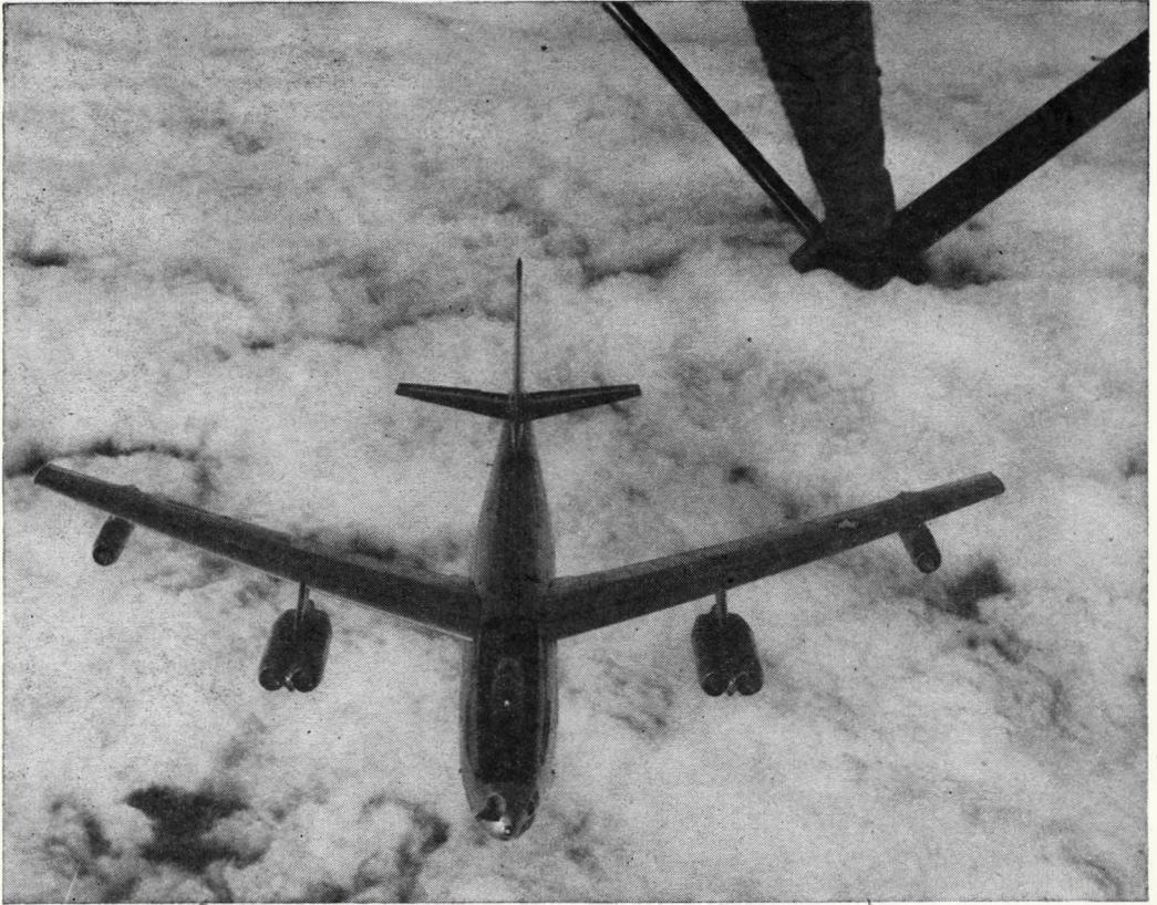
**Refueling in the air: Flying slightly below and behind the Stratotanker (top right), the bomber to be fueled eases its nose toward the flying tanker's tail. When the planes are in position, the Stratotanker's boom operator carefully lowers the telescoping boom, through which the gasoline is hosed, to the receiving receptacle in the bomber (opposite page). If badly handled, the boom could smash the bomber's canopy, wrecking its air-pressure system.**
